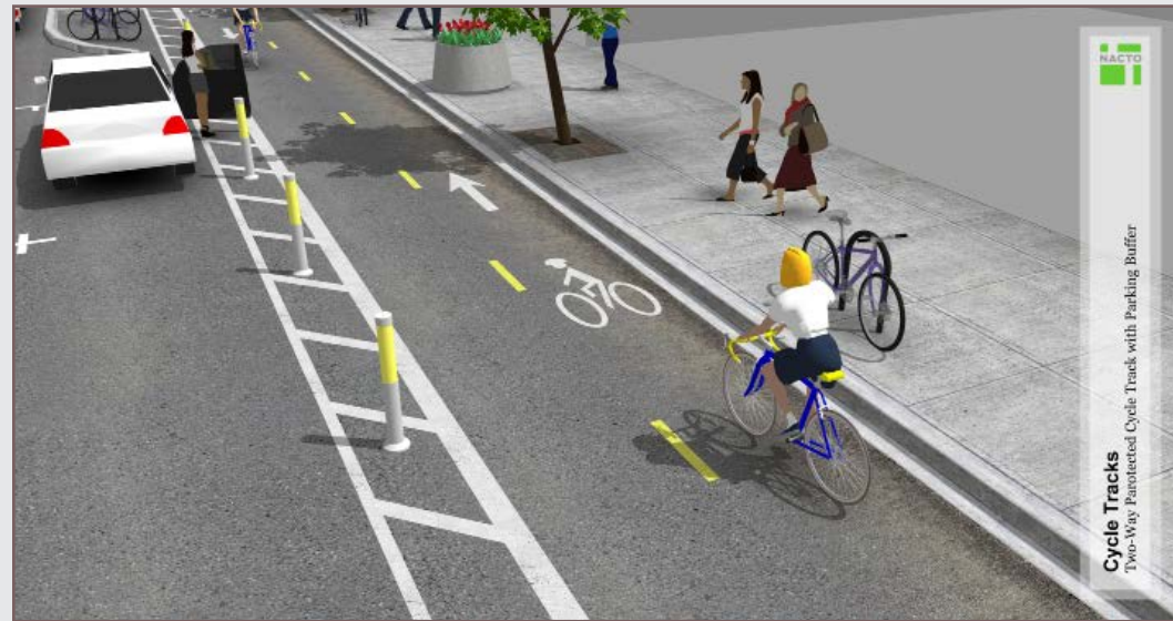
Photo: Example of a buffered cycle track from the NACTO Urban Bikeway Design Guide
