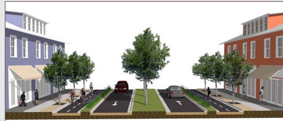
Exhibit III-25: Conceptual Cross Section of Cycle Track
