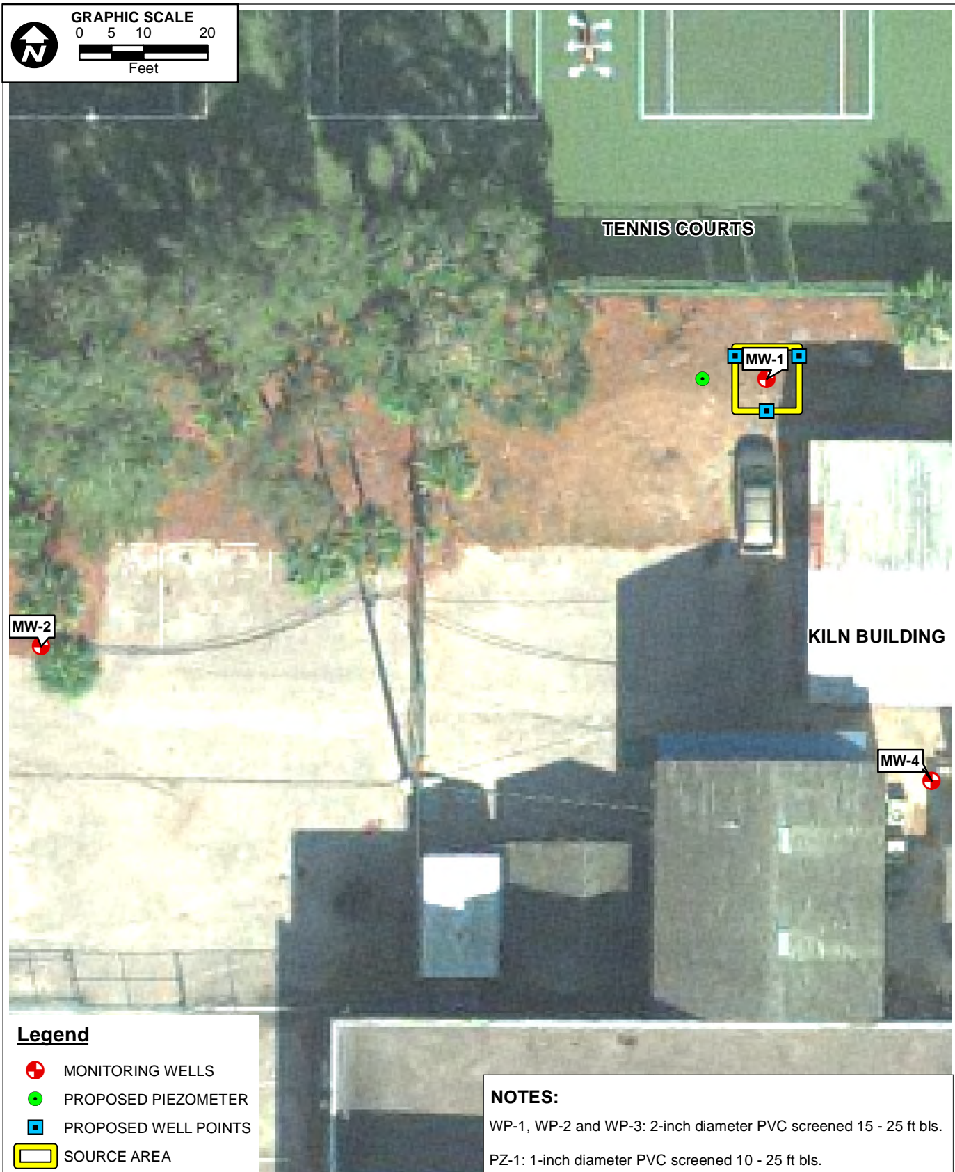
FIGURE 6. PUMP AND TREAT DESIGN PLAN ORLANDO DOWNTOWN RECREATION COMPLEX & TENNIS CENTRE CITY OF ORLANDO, ORANGE COUNTY, FLORIDA SECTION 26, TOWNSHIP 22S, RANGE 29E
