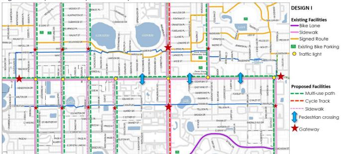
Design I shows sidewalks and multi-use paths along all major east-west and north-south roads, and a two-way cycle track on the east side of Conway Road (see **Figure 9**, Cross-sections). It also shows proposed mid-block street crossings between Conway Gardens Road and Conway Road, between Conway Road and Gaston Foster Road, and between Gaston Foster Road and Dixie Belle Drive.
